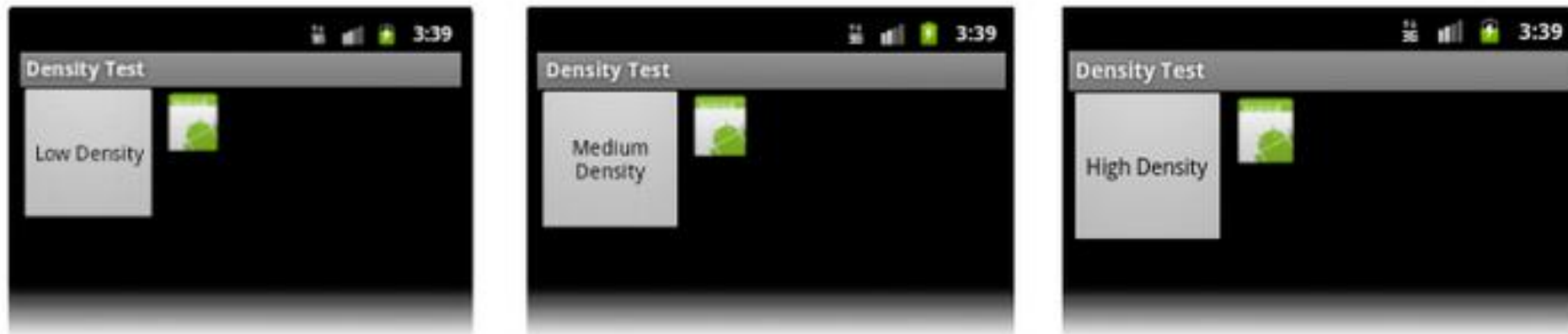
Figure 3. Example application with good support for different densities (it's density independent), as shown on low, medium, and high density screens.
